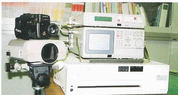
Fig. 8-1. Photograph of the infrared thermal video system. Infrared camera (bottom left), image processor (middle right), real time recorder (top right), handy video camera (top left) and video copy processor (bottom right).
