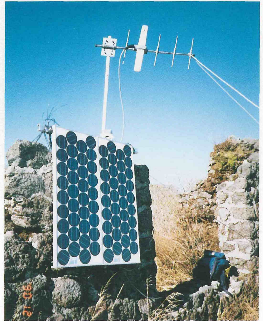
Fig. 7-3. Photograph of the temporary seismic station located at the west rim of the Jigokuato Crater. An antenna of the transmitter and the solar panels can be seen. This station was destroyed and buried by volcanic ash and debris during eruptions of April 1991.
