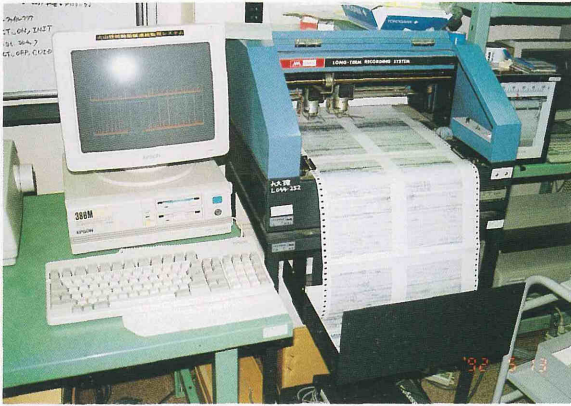
Fig. 7-4. Photograph of the continuous recording system consisting of two 16-channel DAT (Digital Audio Tape) recorders. About one gigabyte of data can be recorded in a small-size cartridge.
