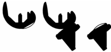
Fig.3 Interpolation by Bezier curvature to restore missing parts of silhouette due to overlapping.
