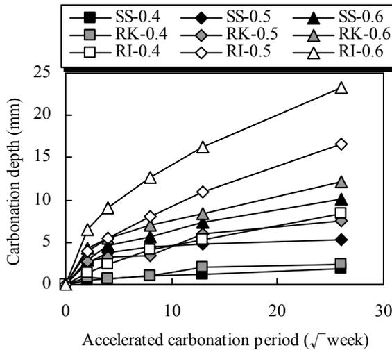
**Fig. 2** Change of carbonation depth of mortar
