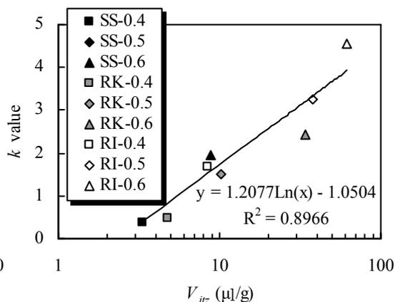
**Fig. 8** Relationship between  $V_{itz}$  and carbonation speed
