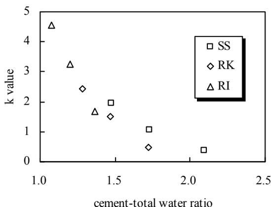
**Fig. 5** Relationship between cement-total water ratio and carbonation
