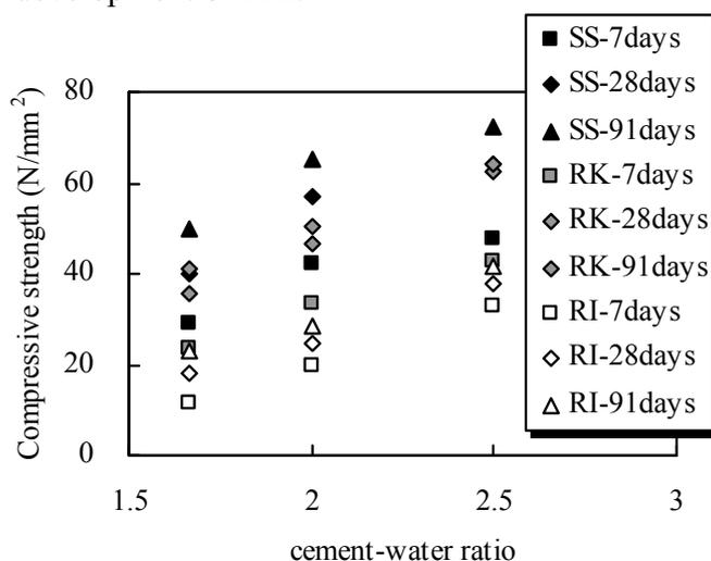
Fig. 1 Relationship between cement-water ratio and compressive strength
