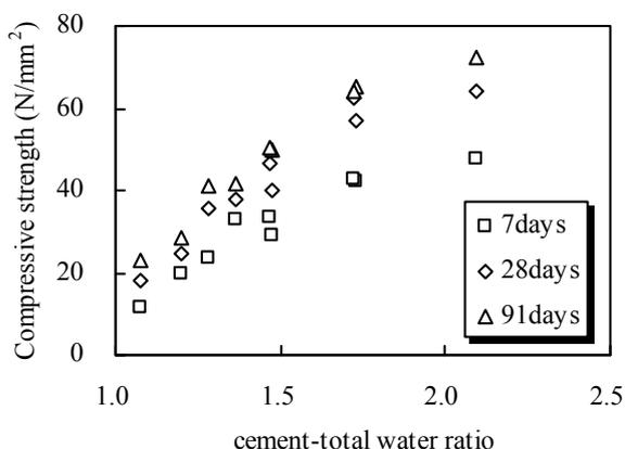
**Fig. 4** Relationship between cement-total water ratio and compressive strength
