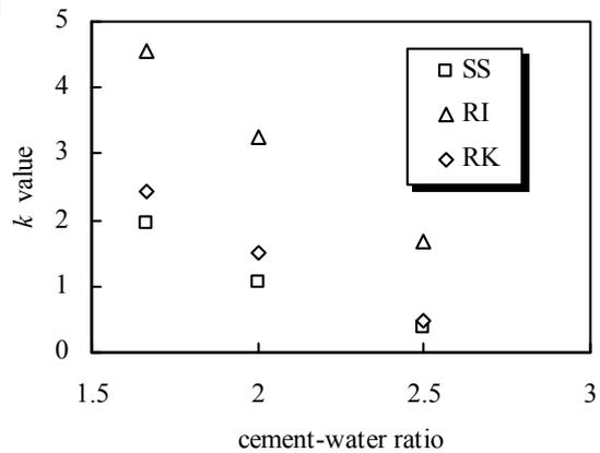
**Fig. 3** Relationship between cement-water ratio and carbonation speed
