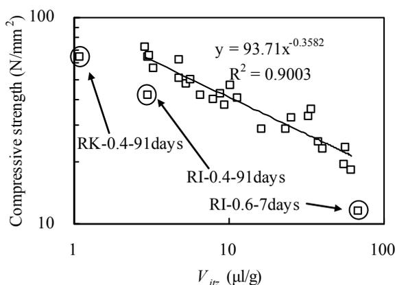
**Fig. 7** Relationship between  $V_{itz}$  and compressive strength
