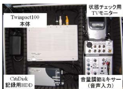
図2. CRP(Contents Recording Package)写真
