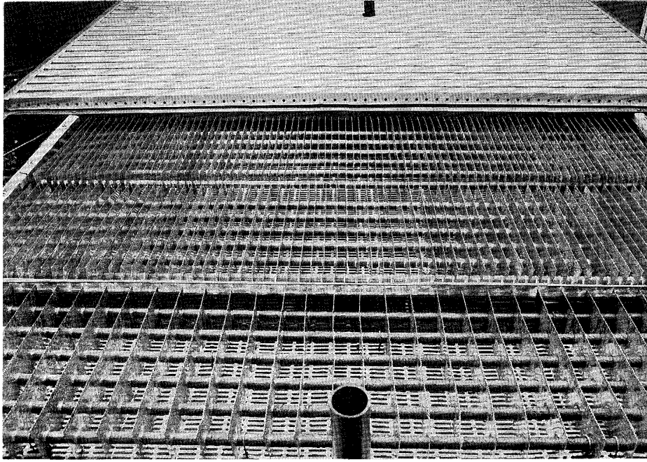
Fig. 2. Supplementary evaporator placed under the plant growth surface, with fins placed at various distances from each other to create a temperature gradient.
