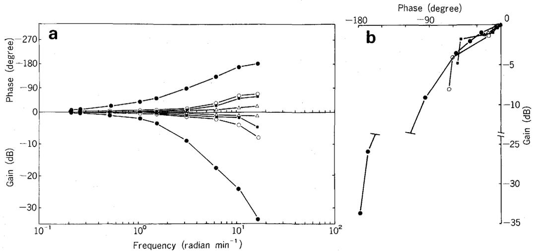
Fig. 13. Frequency responses (a, Bode diagram; b, gain-phase diagram) of sensors to absolute humidity fluctuation at constant air temperature of 25°C and air velocity of 0.6 m sec<sup>-1</sup>: ●, ventilated psychrometer of resistance thermometers; ○, lithium chloride relative humidity sensor; △, electric capacitance meter; ■, absolute humidity sensor of thermistors.
