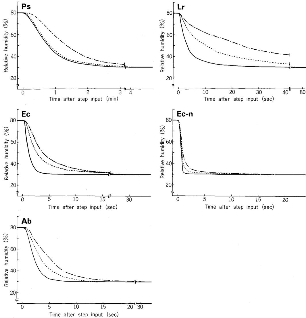
Fig. 4. Step responses of sensors (Ps, Lr, Ec, Ec-n and Ab) to humidity falling (from 80 to 30%RH) at respective air temperatures of 40 (—), 25 (- - -) and 10 (- · - ·)°C and air velocity of 0.6 m sec<sup>-1</sup>: Ps, ventilated psychrometer of resistance thermometers; Lr, lithium chloride relative humidity sensor; Ec, electric capacitance meter; Ec-n, electric capacitance meter (without filter); Ab, absolute humidity sensor of thermistors.
