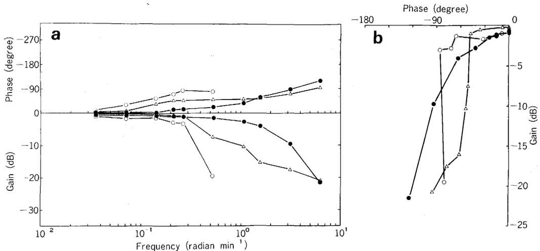
Fig. 14. Frequency responses (a, Bode diagram; b, gain-phase diagram) of sensors to air temperature fluctuation at constant absolute humidity of 14 g m<sup>-3</sup> and air velocity of 0.6 m sec<sup>-1</sup>: ●, ventilated psychrometers of resistance thermometers; ○, lithium chloride relative humidity sensor; △, electric capacitance meter.
