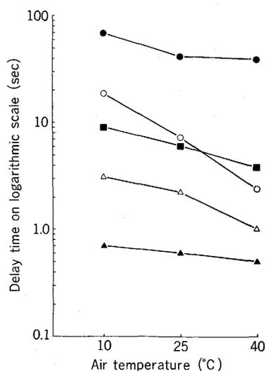
Fig. 5. Relations between air temperatures and delay times in step responses of sensors to humidity falling (from 80 to 30%RH) at air velocity of  $0.6 \text{ m sec}^{-1}$ : ●, ventilated psychrometer of resistance thermometers; ○, lithium chloride relative humidity sensor; △, electric capacitance meter; ▲, electric capacitance meter (without filter); ■, absolute humidity sensor of thermistors.
