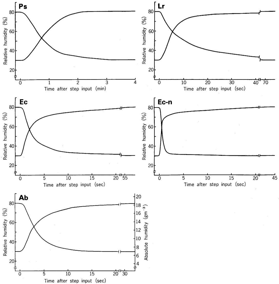
Fig. 3. Step responses of sensors (Ps, Lr, Ec, Ec-n and Ab) to humidity rising (from 30 to 80 %RH) and falling (from 80 to 30%RH) at air temperature of 25°C and air velocity of 0.6 m sec<sup>-1</sup>: Ps, ventilated psychrometer of resistance thermometers; Lr, lithium chloride relative humidity sensor; Ec, electric capacitance meter; Ec-n, electric capacitance meter (without filter); Ab, absolute humidity sensor of thermistors.
