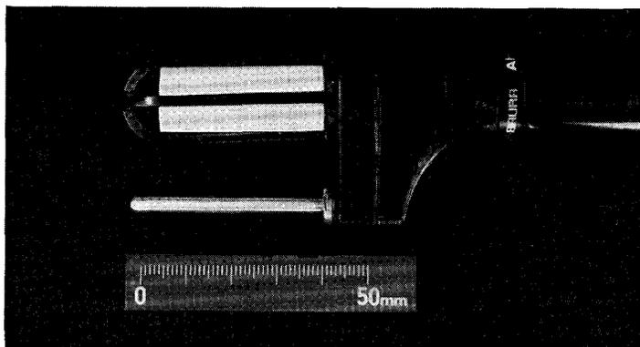
Fig. 1. System diagrams and photographs of ventilated psychrometer of resistance thermometers (Ps), lithium chloride relative humidity sensor (Lr), electric capacitance meter (Ec and Ec-n) and absolute humidity sensor of thermistors (Ab).
