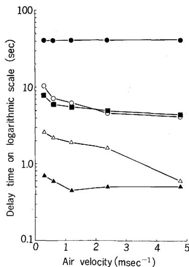
Fig. 7. Relations between air velocities and delay times in step responses of sensors to humidity falling (from 80 to 30%RH) at air temperature of 25°C: ●, ventilated psychrometer of resistance thermometers; ○, lithium chloride relative humidity sensor; △, electric capacitance meter; ▲, electric capacitance meter (without filter); ■, absolute humidity sensor of thermistors.
