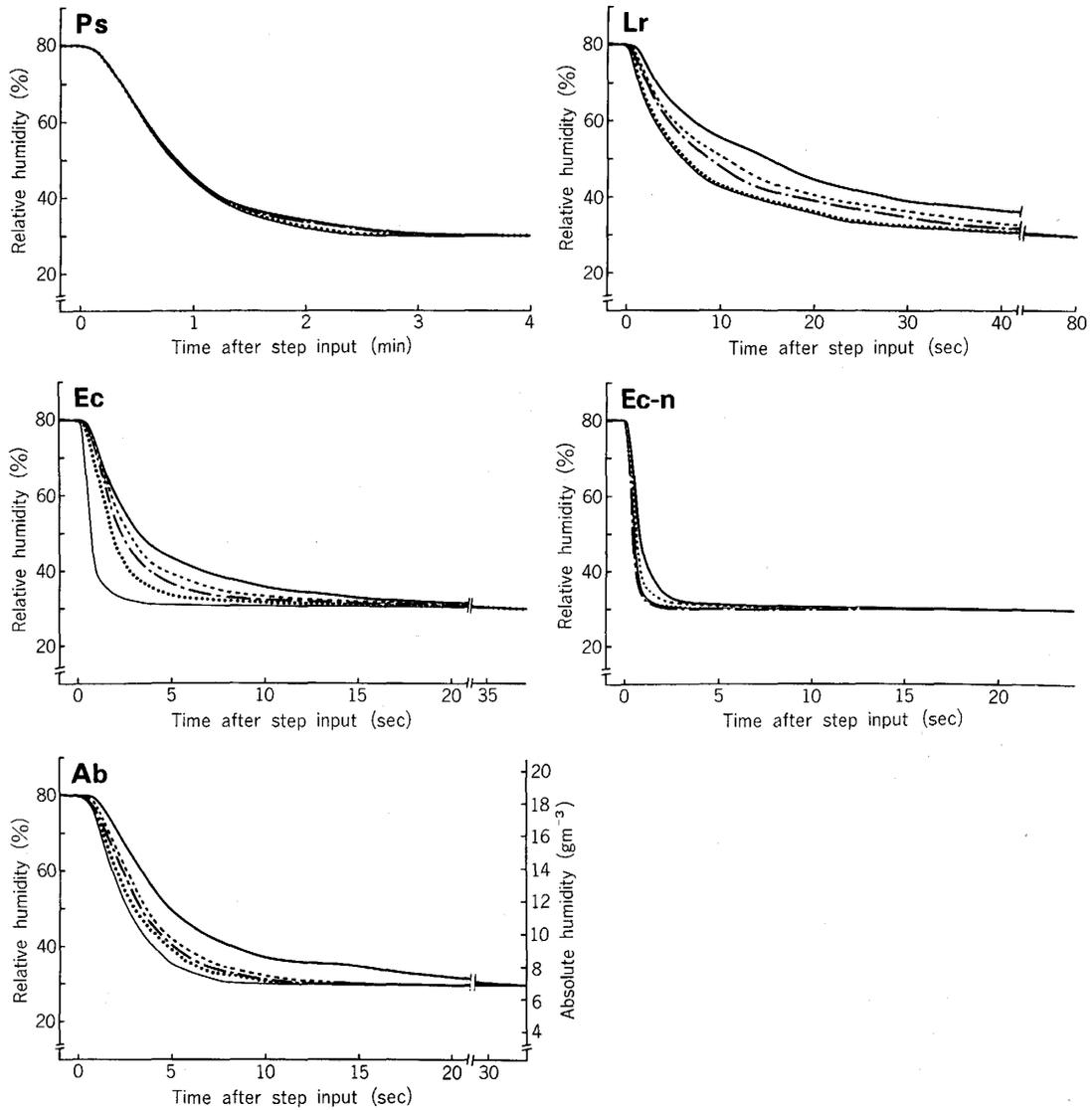
Fig. 6. Step responses of sensors (Ps, Lr, Ec, Ec-n and Ab) to humidity falling (from 80 to 30%RH) at respective air velocities of 4.8 (—), 2.4 (···), 1.2 (---), 0.6 (- · -) and 0.3 (—)  $m\ sec^{-1}$  and air temperature of 25°C: Ps, ventilated psychrometer of resistance thermometers; Lr, lithium chloride relative humidity sensor; Ec, electric capacitance meter; Ec-n, electric capacitance meter (without filter); Ab, absolute humidity sensor of thermistors.
