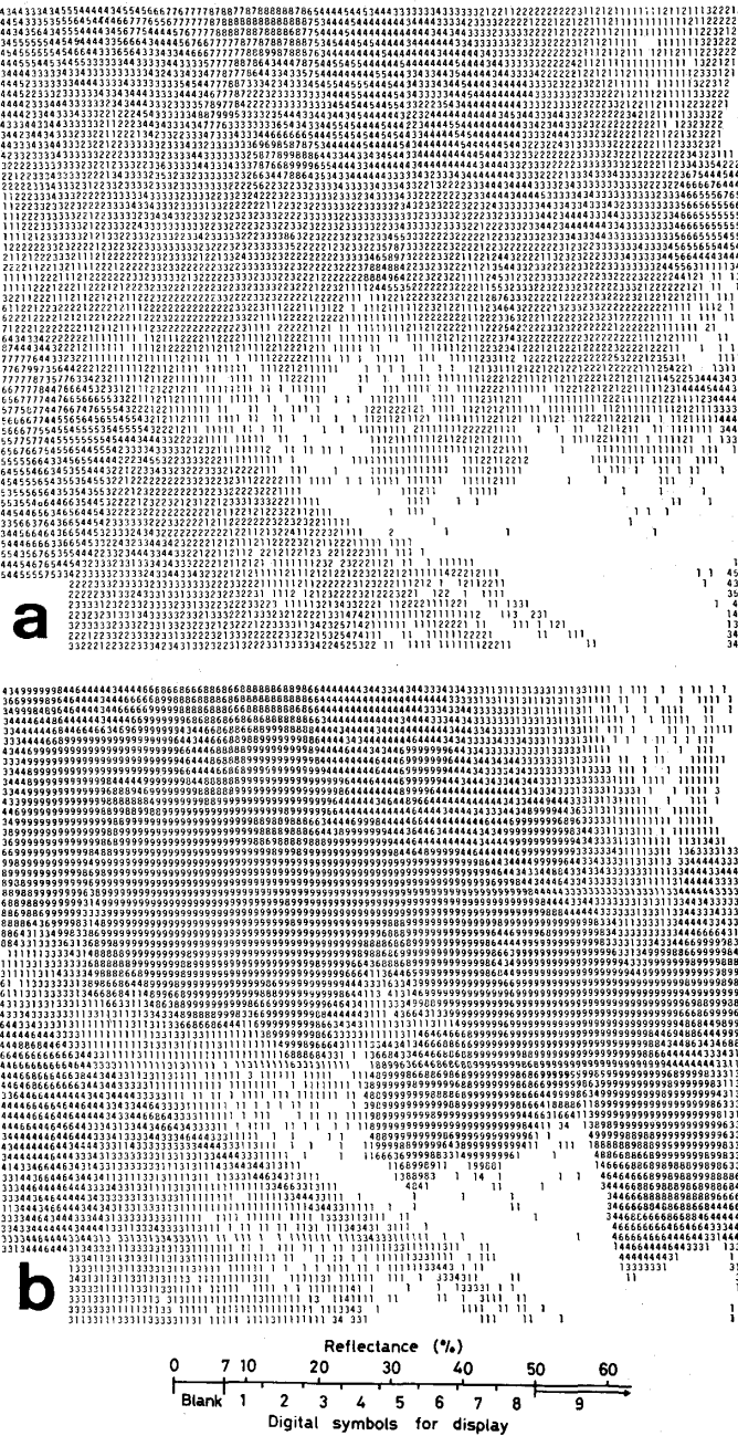
Fig. 6. Digital displays of M_R (a) and M_I (b) derived from R and I images shown in Fig. 5; reflectances are symbolized as illustrated on the scale (odd rows and columns of matrix elements are omitted).
