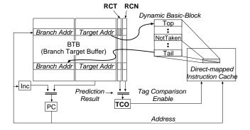
• RCN (Residing in Cache on Not-taken) 1-bit flag per entry: This is an execution footprint for fallthough instructions. This flag is set to 1 when the corresponding branch is not-taken, and is reset to 0 whenever a cache miss or a BTB replacement occurs.
