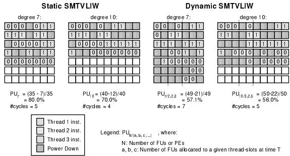
**Figure 2.** According to the influence of the RTOS, different eVLIW inst. may be build for the SSMTVLIW and DSMTVLIW. Thread-slots FU's allotments in the DSMTVLIW may vary during program execution, environment changes or stricter deadlines/power budgets.
