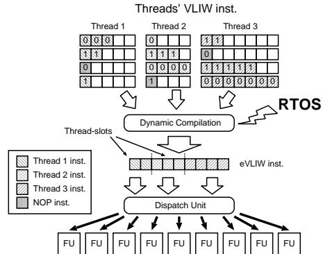
**Figure 1.** The computation model of the SMTVLIW.
