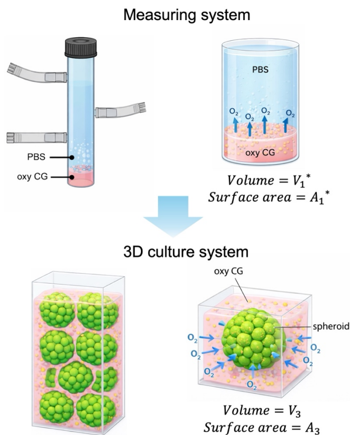
Fig. 5.8 Schematic representation of converting the 2D measuring system to a 3D spheroid–oxy CG culture model for estimating the cultivable cell density threshold. (* the size of hepatocyte spheroid will be shown in Section 5.3.3.1)
