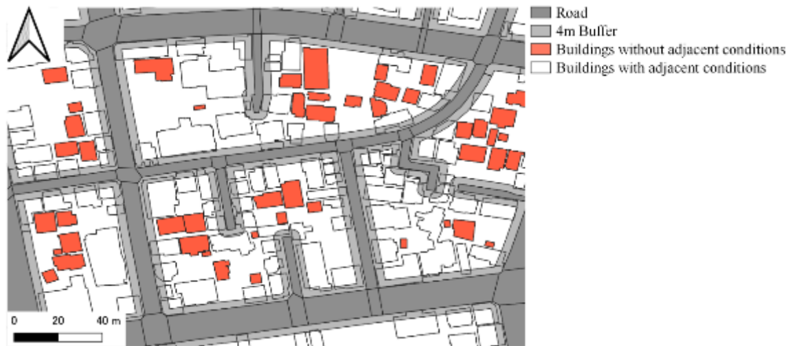
Figure 6.3. Criteria for determining adjacent conditions
