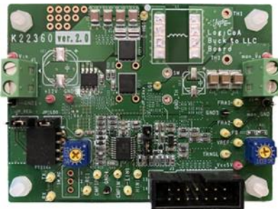
Fig.10. Prototype board of LLC D-EPC
