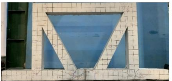
Fig. 9: Crack location of EBFV-25 model
