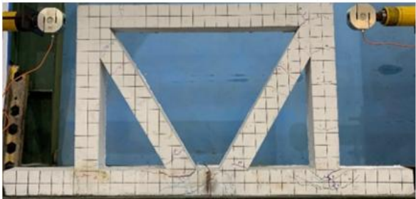
Fig. 8: Crack location of EBFV-15 model
