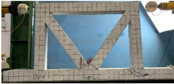
Fig. 7: Crack location of CBF model
