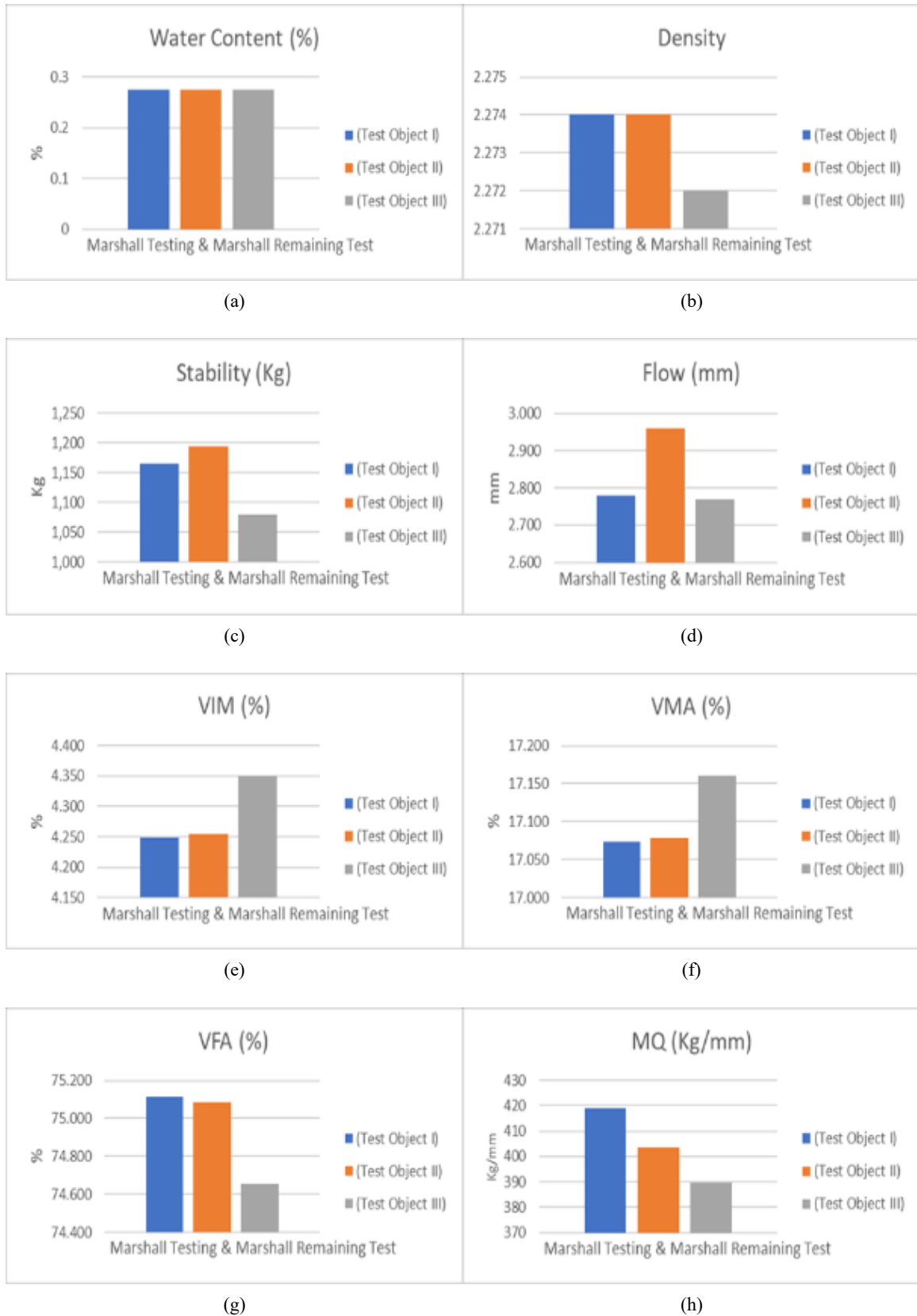
Fig. 7: Marshall Characteristic Test Chart, (a) Water Content, (b) Density, (c) Stability, (d) Flow, (e) VIM, (f) VMA, (g) VFA, (h) MQ
