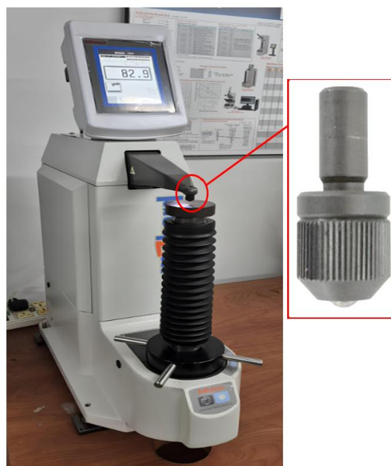
Fig. 3: The Rockwell hardness testing machine was used to evaluate hardness according to the HRL scale with a 6.35 mm steel ball indenter
