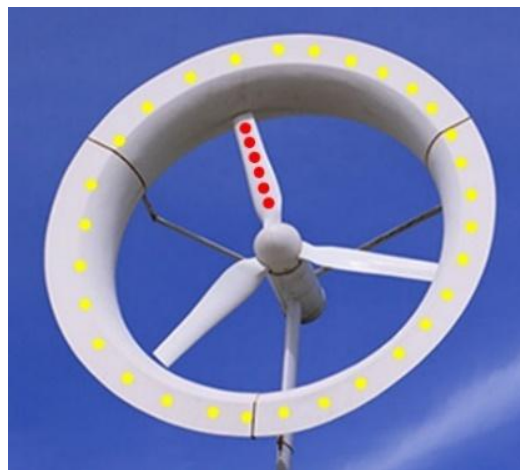
Fig. 3: Actuator representation of the rotor and diffuser
