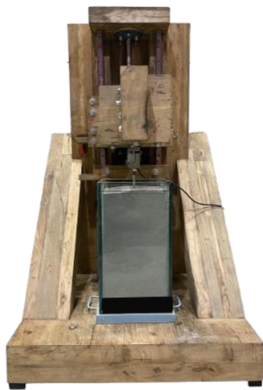
Fig. 6: Automatic Small-Scale Compression Testing Equipment with Data Logger
