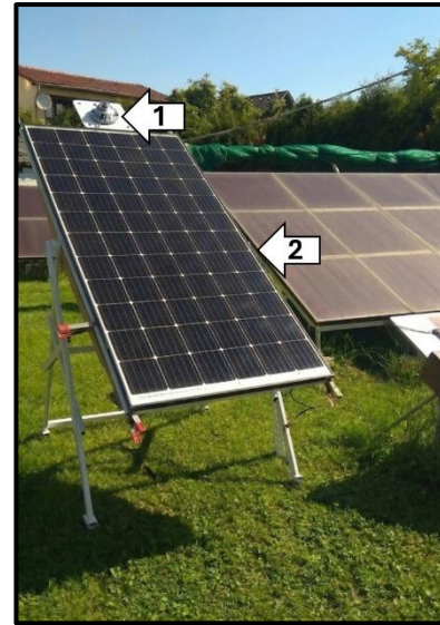
Fig. 3: The measurement setup of the bifacial PV module under real environmental conditions (1: Hukseflux LP02 pyranometer; 2: JA Solar JAM72D00-370/BP PV module)
