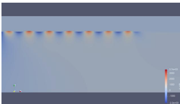
(c) The pressure distribution in the viscous-NWT
