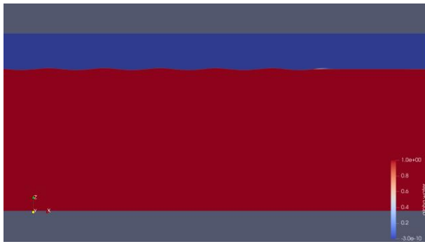
(a) The free-surface deformation in the viscous-NWT
