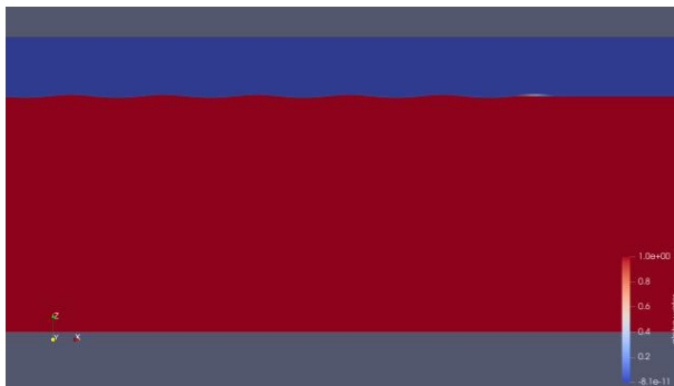
(a) The free-surface deformation in the viscous-NWT
