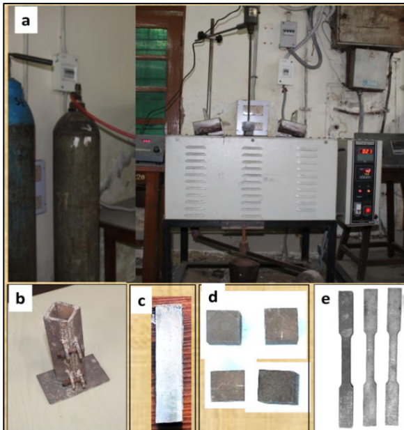
Fig.1: (a) stir casting setup (b) Mold of cast iron (c) as cast sample (d) prepared sample for optical microscopy and Vickers hardness study (e) Tensile sample
