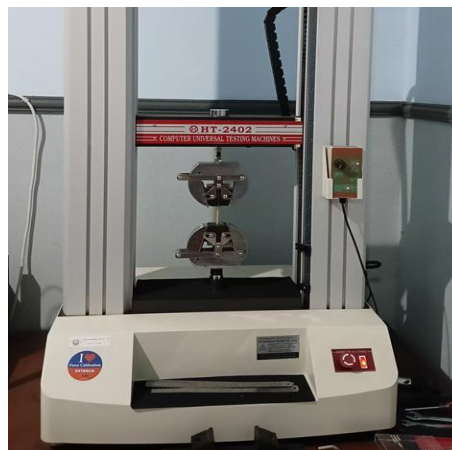
Fig. 3: Tensile test setup (HT-2402 UTM)
