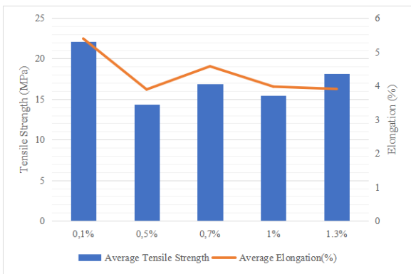
Fig. 5: Tensile Strength and Elongation Result in Catalyst Variation
