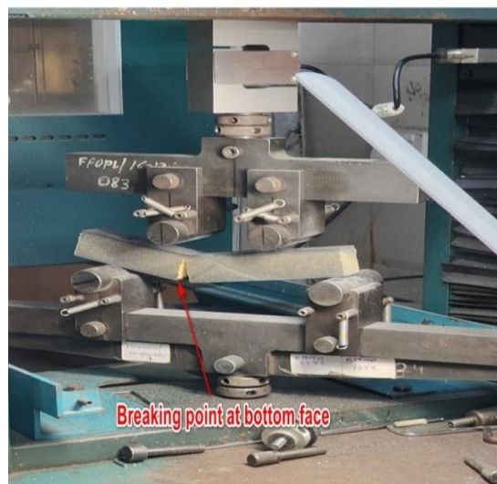
Fig. 15: Breaking point of carbon fiber (top 4 layers bottom 2 layers) sandwich composite
