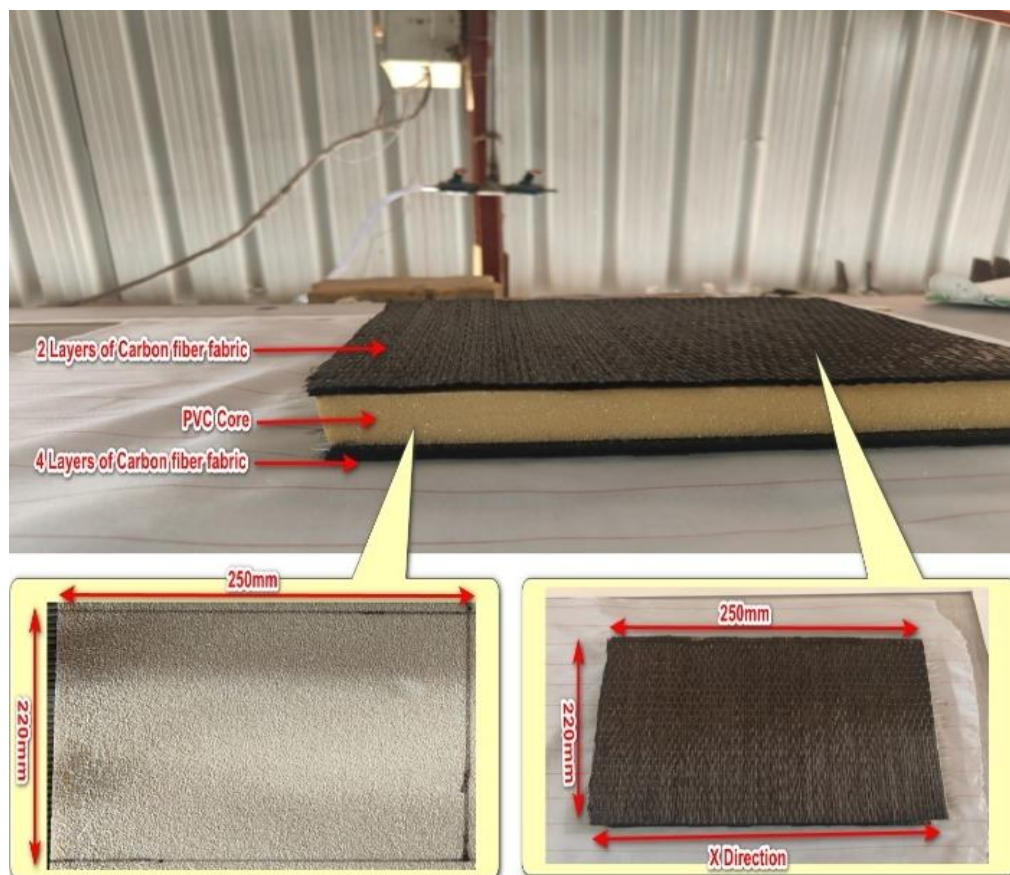
Fig. 2: Carbon fabric and PVC core setup
