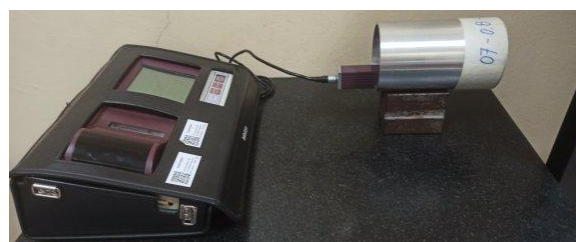
(b) SR measurement using Mitutoyo SJ-301 Fig. 5: Measurement Instrument
