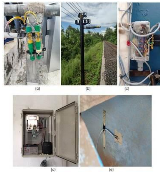
Fig. 5: (a) subsidence sensor; (b) PIR sensor; (c) modbus controller; (d) data logger; (e) strain gauge sensor
