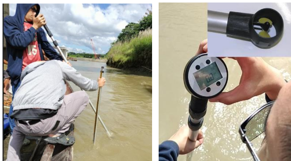
Fig. 7. Field verification survey for computing independent discharge data. A stadia rod (left) and flow probe (right) were used to measure the depth and stream velocity, respectively.
