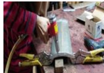
Fig. 7. Riveting process on blades used an air rivet.
