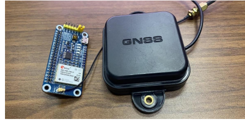
Figure 14. Zed F9P RTK for GNSS tracking
