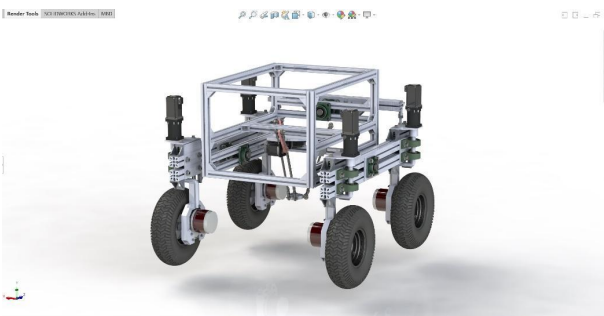
Figure 3. Modular design of the UGV that can accommodate different payloads depending on the mission set.
