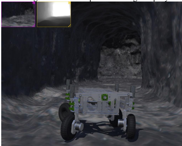
Figure 17. Mine GEARS UGV underground tunnel navigation simulated in Webots
