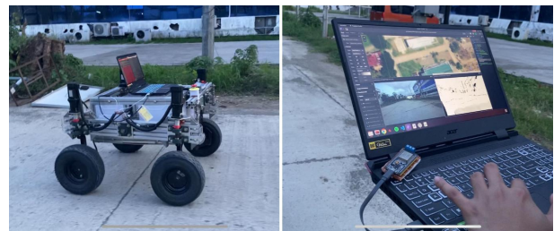
Figure 15. Zed F9P RTK tested with the UGV for waypoint navigation.
