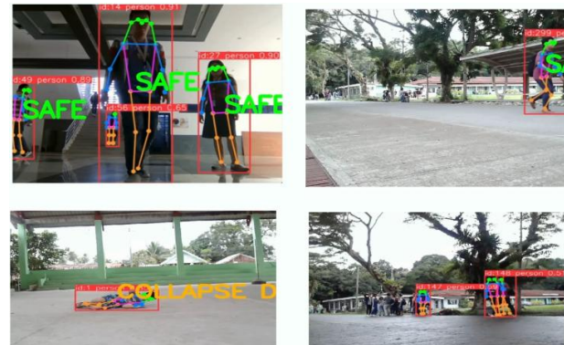
Figure 21. Collapse detection system integrated in the Mine GEARS software stack
