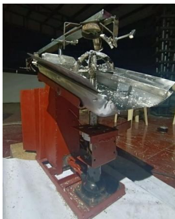
Fig. 7. Fabricated Semi-Automated Coconut Grater Machine during Testing
