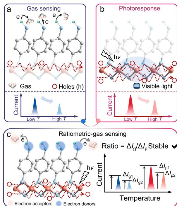
Fig. 6: (a) The gas sensing response process. (b) The photo-response process. (c) The ratiometric gas-sensing detection. Ag: red; S: blue; C: gray; H: green. The figure is used under a Creative Commons Attribution-NonCommercial-NoDerivatives 4.0 International License (CC BY-NC-ND 4.0) [59].
