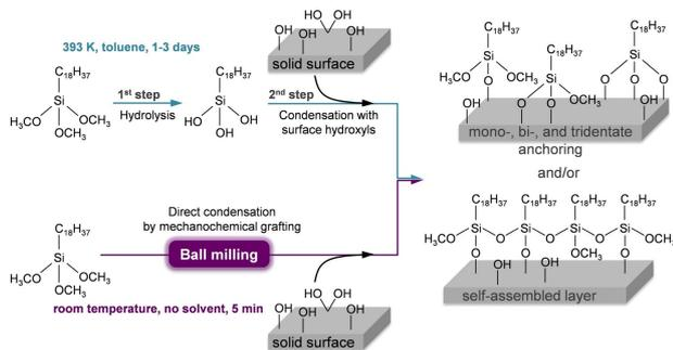
Fig. 2: Schematic representation of hybrid inorganic–organic material synthesis by chemical grafting via the conventional solvothermal route (top) versus solvent-free mechanochemical synthesis (bottom) shown for the functionalization of solids by octadecyltrimethoxysilane (OTMS). Copyright © 2020 American Chemical Society. This publication is licensed under CC-BY [21].
