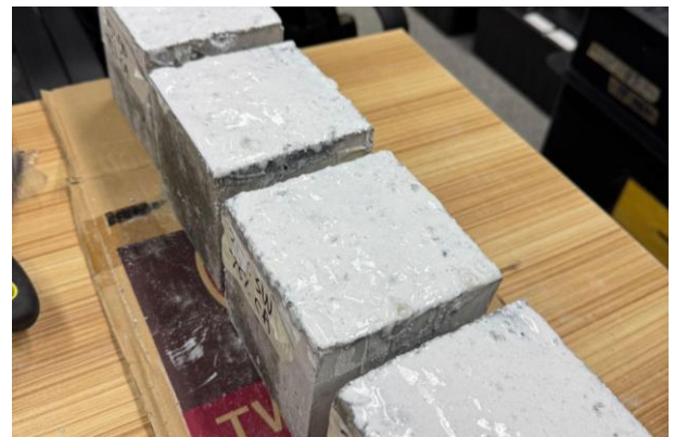
Fig.7. Application of Coating to Concrete Specimens
