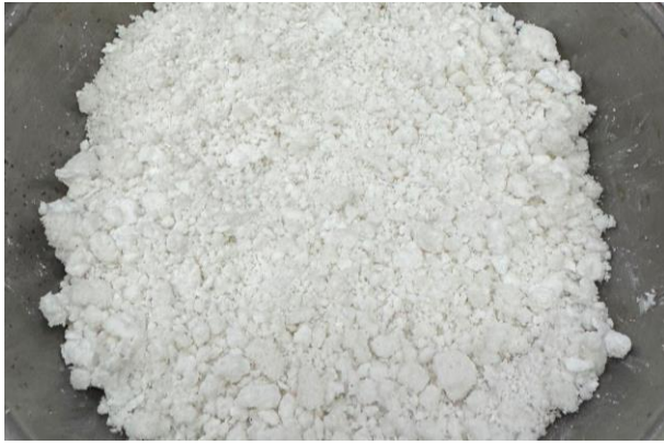
Fig.4. Mg (OH) 2 derived from Natural Seawater
