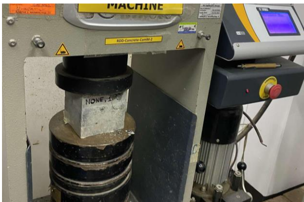
Fig.9. Compressive Strength Test using UTM
