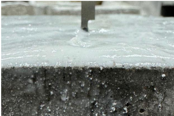
Fig.8. Verification of Coating Thickness on Concrete Specimens
