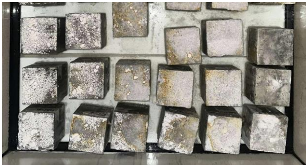
Fig. 11. Concrete Cubes After 4 Days of Sulfuric Acid Exposure
