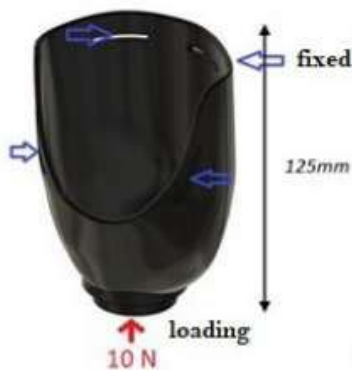
Fig. 1. 3D printed hand orthosis for upper limb [8]
