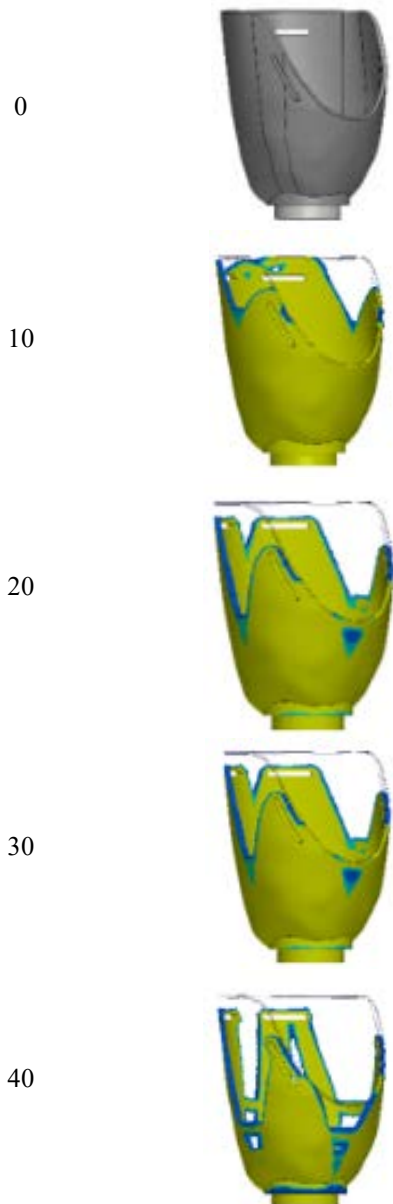
Topology optimization (%) Hand orthosis based on weight reduction
