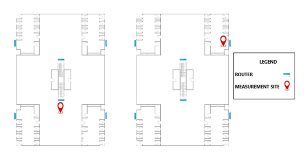
Fig. 1. On the left side is the floor plan of second floor at Blok C and on the right side is the floor plan of fourth floor at Blok M. The point of measurement is marked using a red pin on the plan. The blue colored symbol on the plan represents a router.
