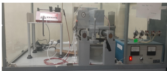
Fig. 1. Electrospinning setup used in the study.
