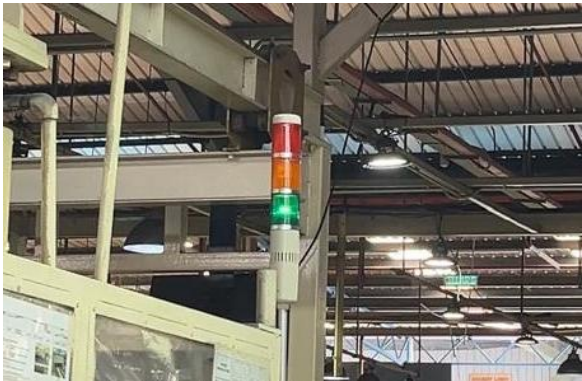
Fig. 10. Tower lights indicator for the system
