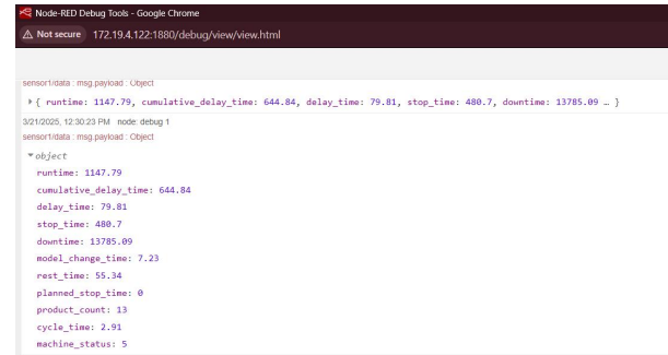
Fig. 5. Data displayed in Node-Red sent using MQTT
