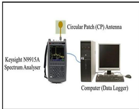
Fig. 1. Measurement Setup using Circular Patch Antenna, Spectrum Analyser, and Data Logging System
