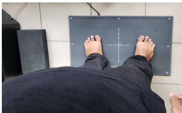
Fig. 3 : The starting position of the bipedal standing test. Each subject was instructed to remain stationary with barefoot for 40 s during the trial.
