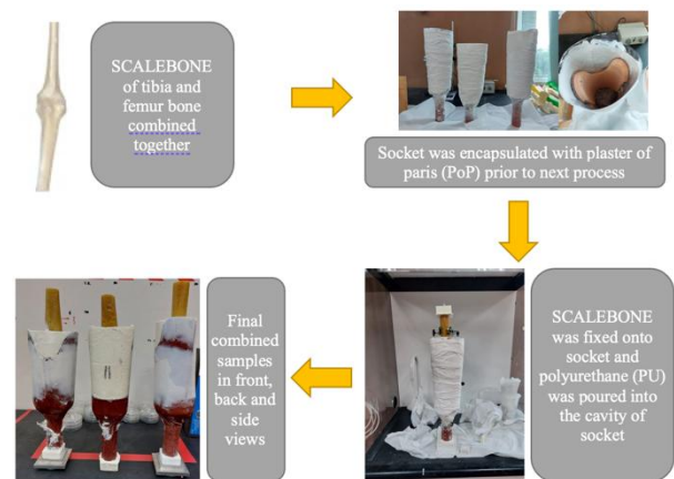
Fig. 2. A flow that illustrated the process of developing mock residual limb.
