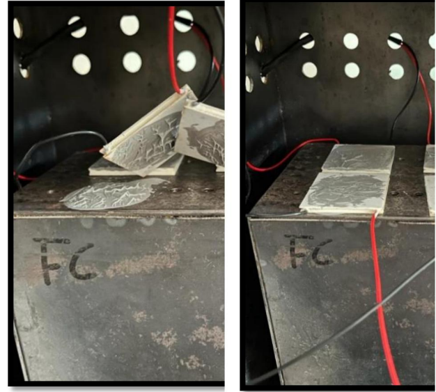
Fig. 3. (a) Thermal Paste Applied on Hot Side of TEG (b) Thermal Paste Applied on Cold Side of TEG
