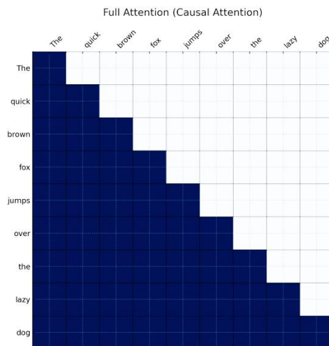
Fig. 1. Causal Full Attention Connectivity Matrix with Lower-Triangular Masking for Token Dependency Control
