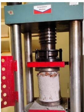
Fig 2.6 Compressive Strength Test
