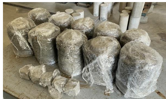
Fig 2.4 Plastic Sheet Curing of Confined and Unconfined Cylinders
