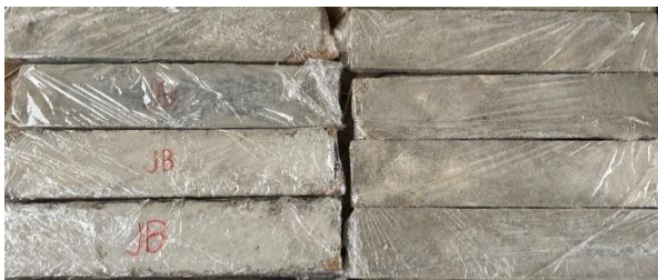
Fig 2 Plastic Sheet Curing of TRM coupons
