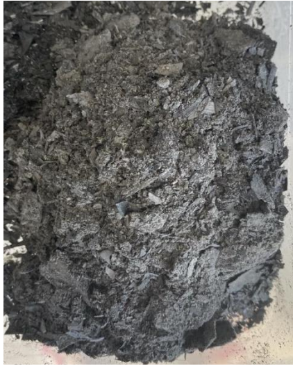
Fig. 1. BLA burned for 2 hours at 400°C
