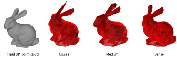
Fig. 3. Reconstructing a bunny in Raspi4. Left: input 3D point cloud. Right: reconstructions with increasing mesh complexity.
