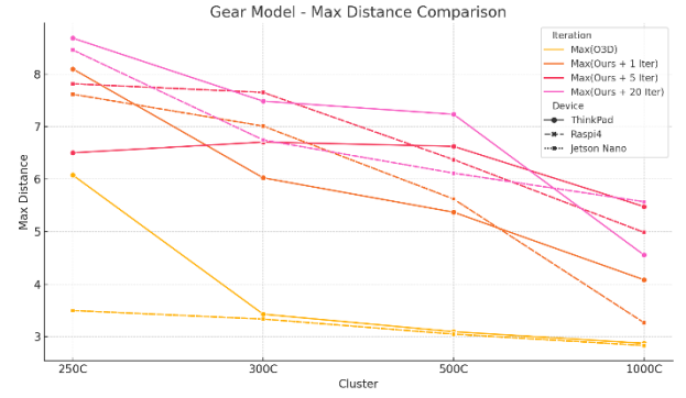
Fig. 18. Maximum distances from 3D input clouds (Gear model) to output meshes in Lenovo ThinkPad, Raspberry Pi 4, and Jetson Nano. Open3D followed VSA-QEM
