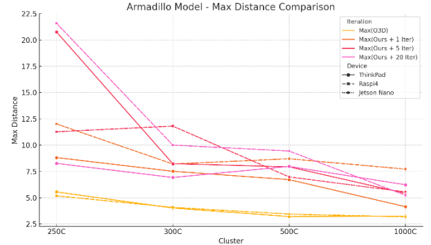
Fig. 20. Maximum distances from 3D input clouds (Armadillo model) to output meshes in Lenovo ThinkPad, Raspberry Pi 4, and Jetson Nano. Open3D followed VSA-QEM
