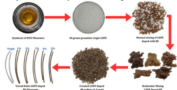
Fig. 3. Illustration of the LDPE-BE Composite Filament Fabrication Process.
