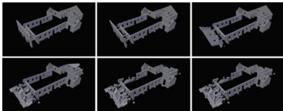
Fig. 6. Simulated structural response of the Parish Church of Santa Monica at Intensity IX using Blender.
