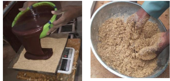
Figure 4: Mixing of Gum Arabic by weight of Rice husk.
