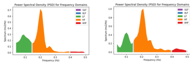
Fig. 11. HRV analysis during exposure to neutral visual stimuli (left: ECG-derived signal, right: textile sensor-derived signal)
