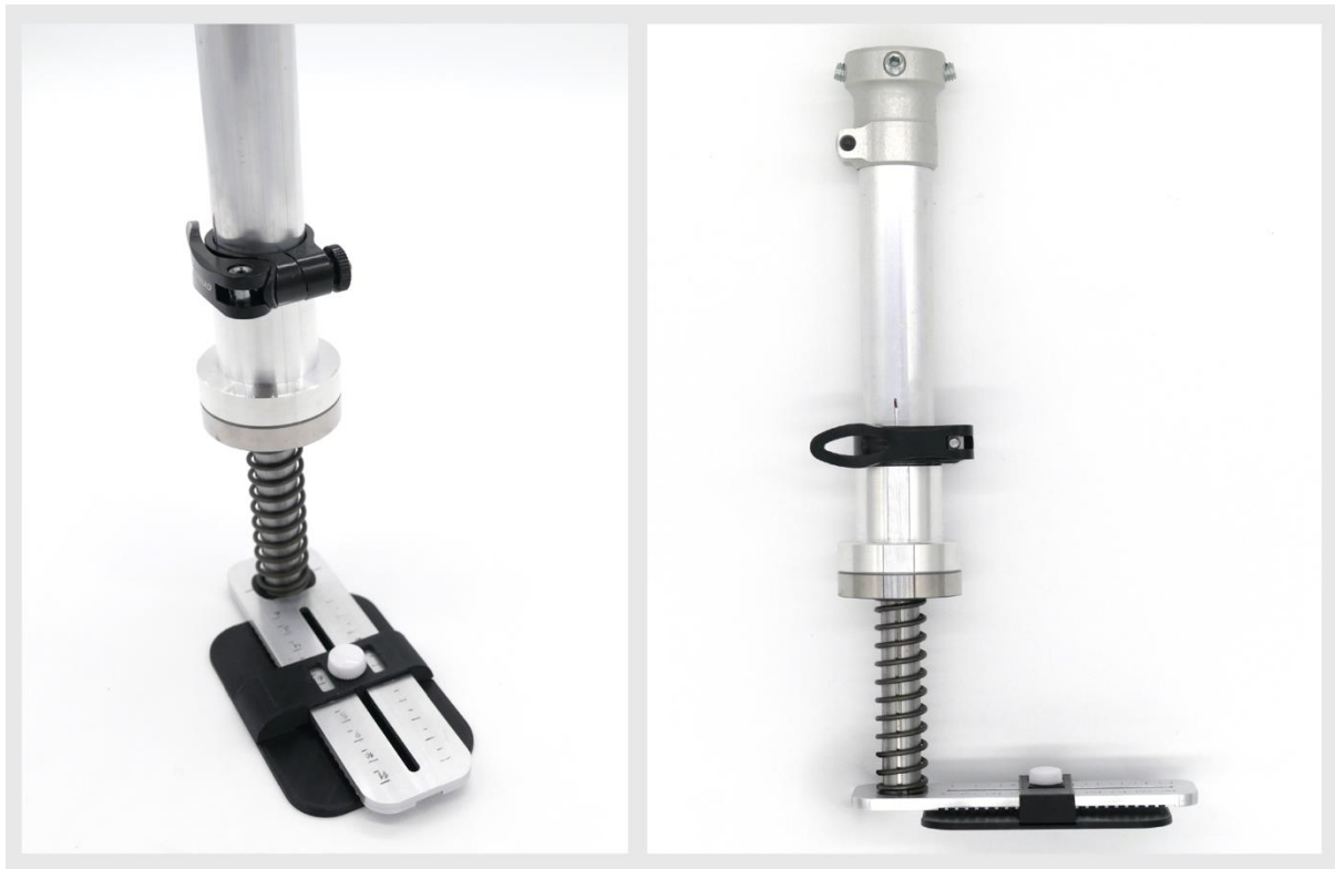
Figure 3.5. Prototype prosthesis fitted with the soft spring.
