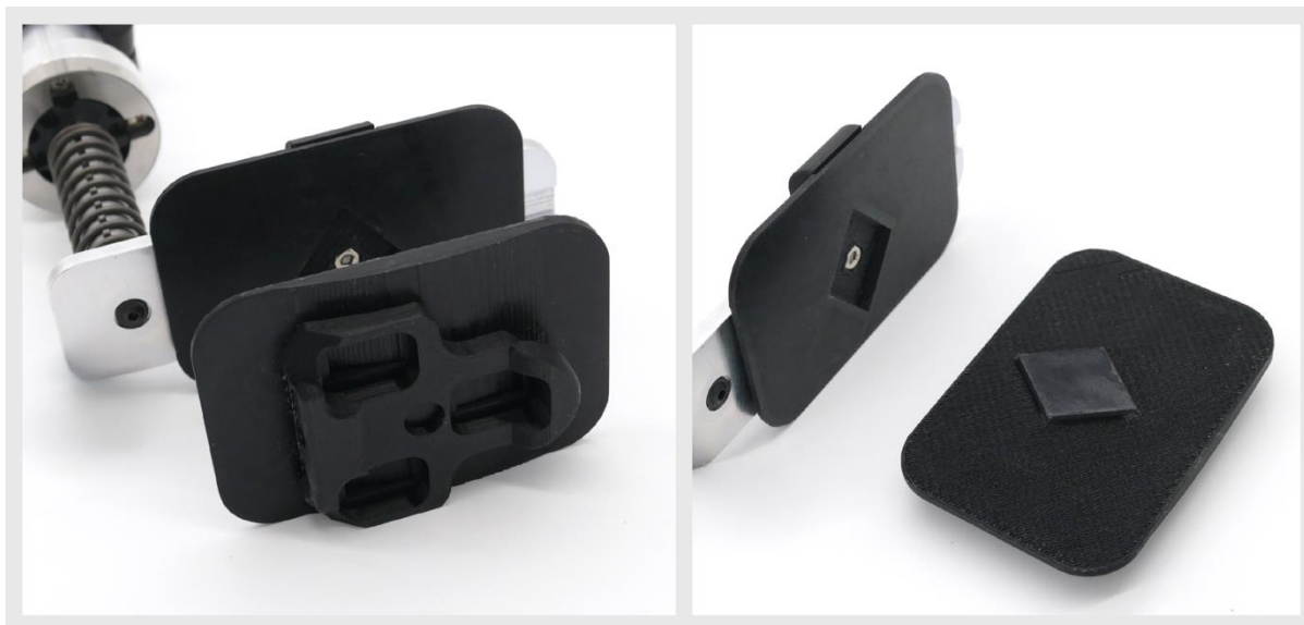
Figure 3.4. Plates used to control the positioning of the foot on the pedal. A diamond shape present in the pedal cleat fitted into a plate on the prosthesis. This plate was also used in the unaffected leg.
