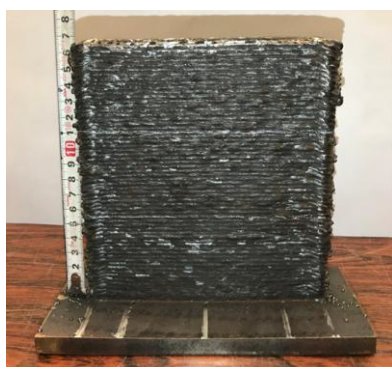
Fig. 1 Appearance of a wall with 120 layers deposited by CO 2 gas shielded arc welding.
