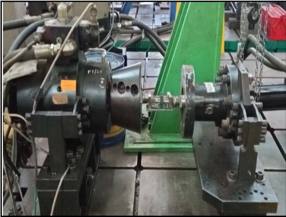
Fig. 6: Test Rig for Gear Pair
